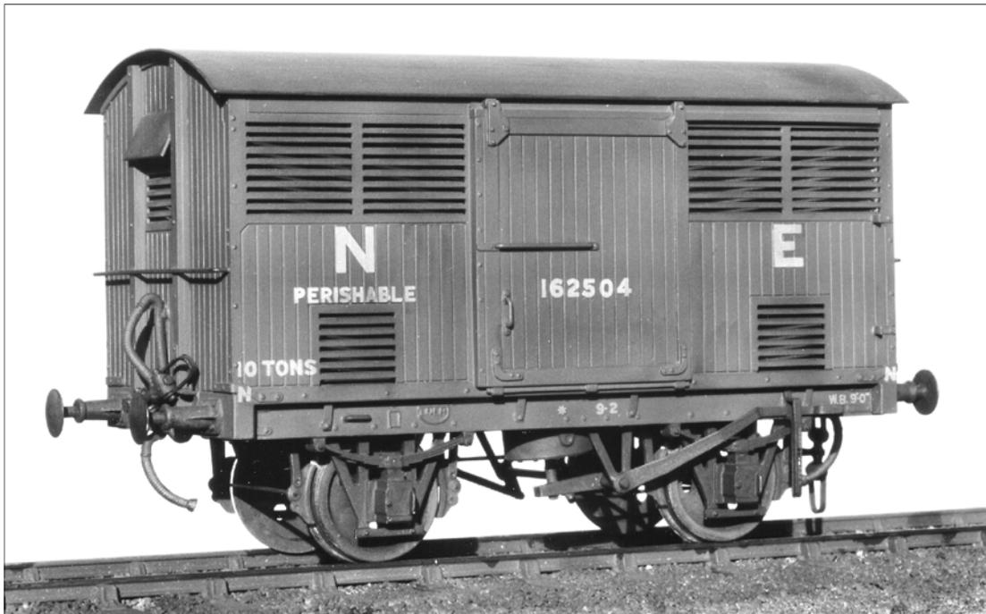
**Prototype.** These vans were a sliding door development of a NER design built by the LNER. They had louvered sides and ends to create a through flow of air to keep the perishable goods such as fruit and vegetables in good condition. This traffic was moved with the utmost haste and the vans were fitted with vacuum brake and through steam pipes to enable them to run in passenger trains.
